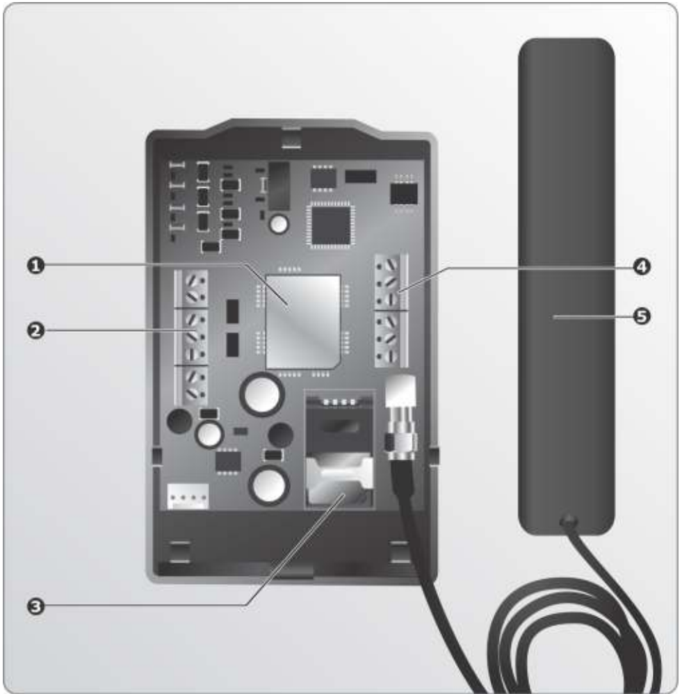
FIGURE 3. GSM CONTROLLER INTERIOR
